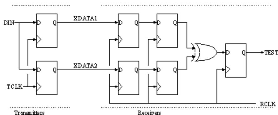
Every once in a while TEST is observed to be "1" for one period of RCLK. Give a brief explanation of why this happens. You can assume that DIN is meeting the setup time of the transmitter registers and that the value for DIN changes much less frequently than TCLK/RCLK. Hint: it has nothing to do with the register that was added to deglitch the TEST output. Think about what's happening in the two pulse synchronizers and why they might generate different outputs for a single clock cycle.
