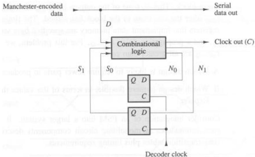
The combinational portion of the decoder has as inputs the Manchester-encoded signal and the current state of the two flip-flops. The combinational logic outputs the next state  $N_1$  and  $N_0$  for the two flip-flops and the clock signal  $C$  generated for the stream of serial data. The truth table of the combinational logic is as follows:
