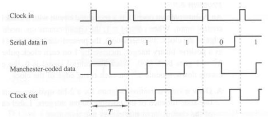
The period of the "decoder clock" that drives the D flip-flops need not be  $T$ ; in general, it will be faster.
